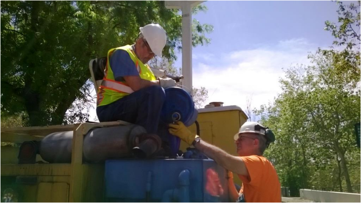
Ed and Dave add hydraulic fluid to the man-lift
